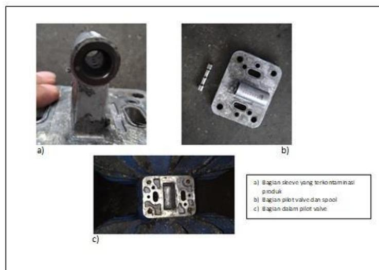
Gambar 4. Overhaul Pilot Valve
